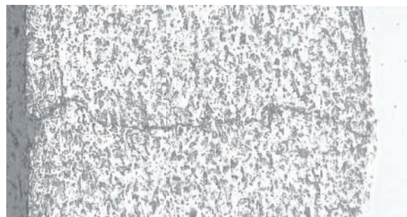
Fig. 6. Fatigue crack of alloy layer (cross-section, enlargement 300x)
